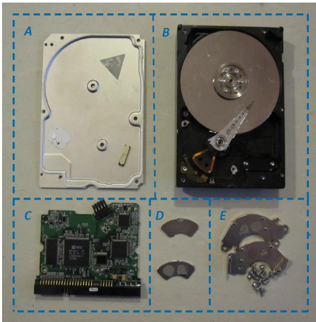
Figure 7 Dismantling depth of the hard disk drive
